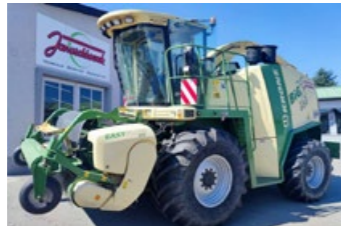
Krone BIG X 650 (653 PS) Bj 2007 3.404 h, 161 MB V8 Motor, 28 Messer Trommel, PickUp 3001 - 3 m, Easy Collect 7500 2-teilig - 10 Reihler, 40 km/h, ... Preis inkl. 20 % MWSt. EUR 118.680,-
