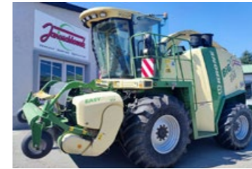
Krone Big X 650 (653 PS) Bj 2007 3.404 h, 16 l MB V8 Motor, 28 Messer Trommel, PickUp 3001 - 3 m, Easy Collect 7500 2-teilig - 10 Reiher, 40 km/h, ... Preis inkl. 20 % MWSt. EUR 118.680,-
